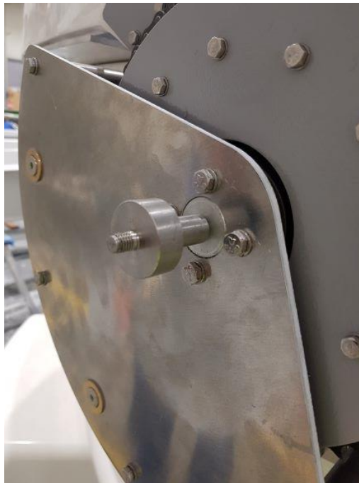
Figure. 60 – Mounted spacer bolt in the main shaft hole.
