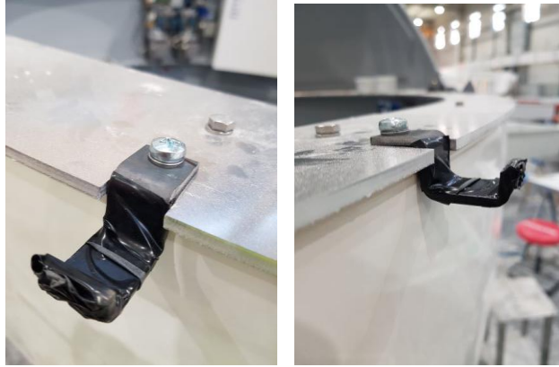
Figure. 46 – Attached Parking Handles for mounting shutter No. 2
