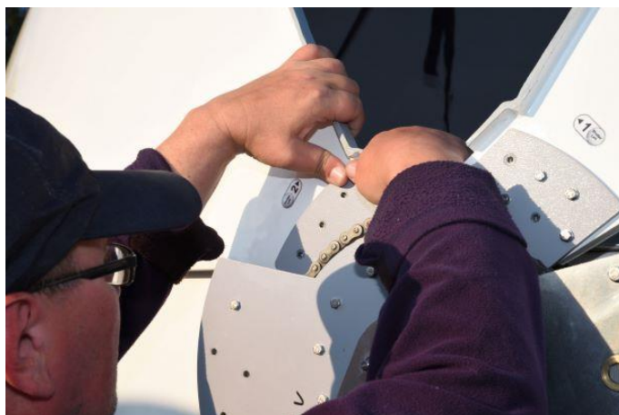
Figure. 48 – Setting shutter No. 2 in the holder
