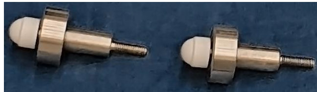
Figure. 59 – Spacer screws for fixing the covers of external drive units.
