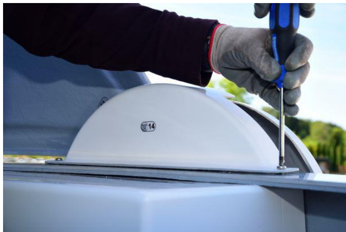
Figure. 58 – installation of the gear inner cover
