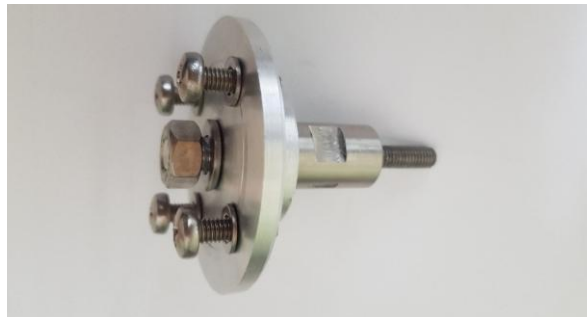
Figure. 59 – Spacer screw for fixing the covers of external drive units.
