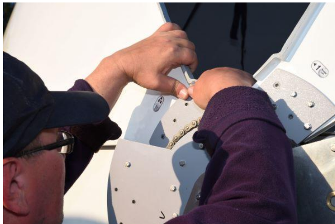
Figure. 48 – Setting shutter No. 2 in the holder
