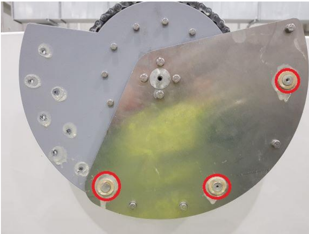
Figure. 75 –Axle tip bearing lubrication points
