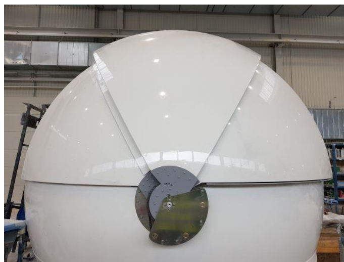
Figure. 56 – observatory with shutters installed in closed position
