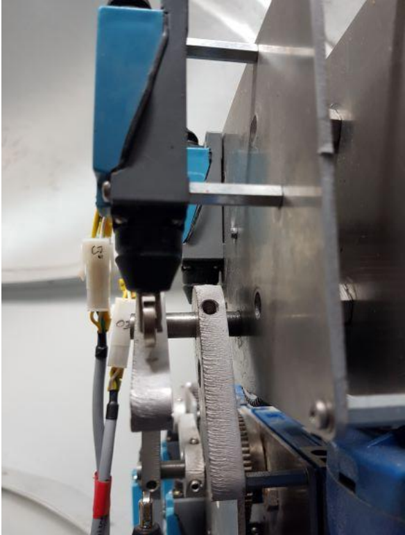
Figure. 74 – View of the end switch and its pusher while acting with pusher
