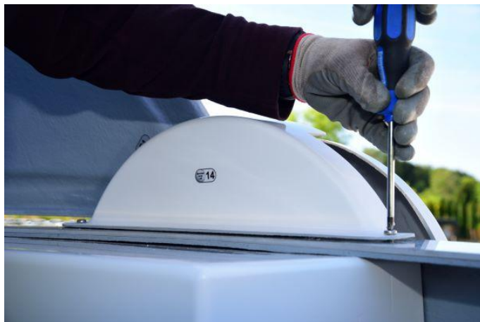
Figure. 58 – installation of the gear inner cover
