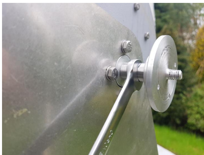
Figure. 60 – Mounted spacer bolt in the main shaft hole.
