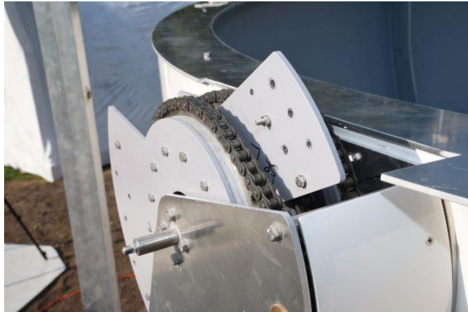
Figure. 38 – washer and fixing screws in the shutter mounting handles and handle position before its installation
