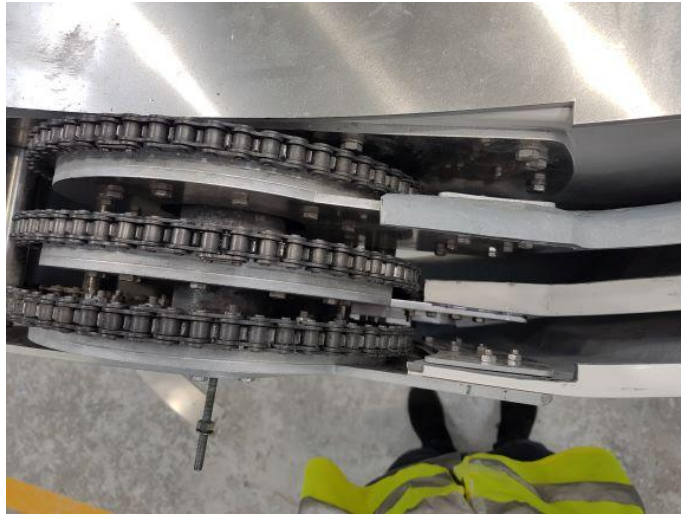
Figure. 57 – position the shutters in the open position of the observatory. From top: shutter #2, shutter #1, shutter #3
