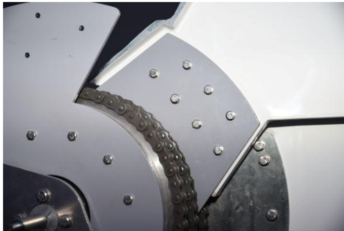
Figure. 48 – Screw connections of shutter No. 2
