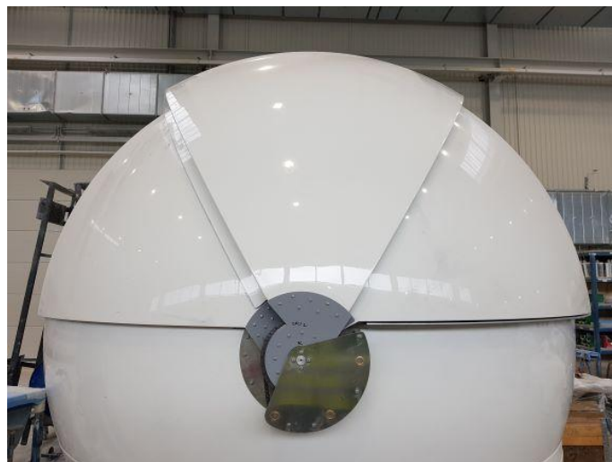
Figure. 56 – observatory with shutters installed in closed position
