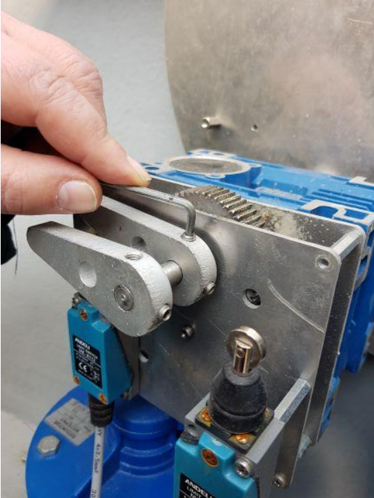
Figure. 73 – View of the end switch and its pusher
