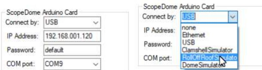
Select the appropriate option in "Connect By" in the Config-> Card-> ScopeDome Arduino Card window.
