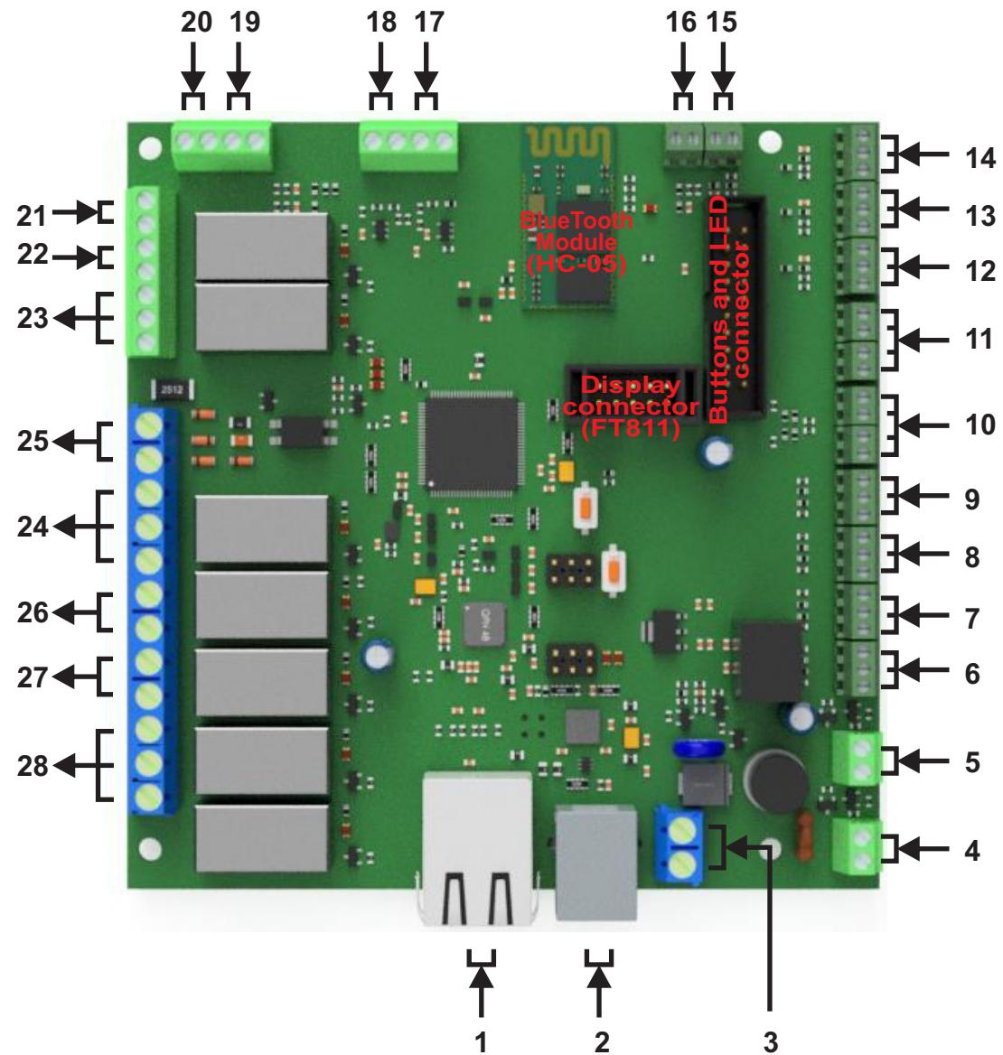
Button and Led Connector - dedicated cards can be connected to this PCB with necessary buttons and LEDs to allow control the relays.
