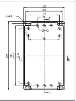
fig. 1 Mounting holes for stationary and rotary part
