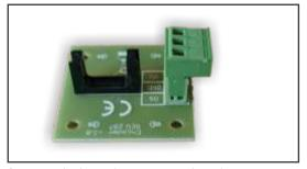
fig. 3 Enkoder and HomeSensor board
