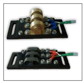
fig. 6 Power contacts for 4M i 55M dome
