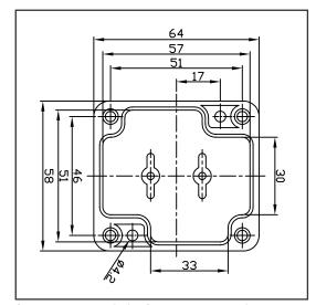
fig. 2 Mounting holes for Higrometer and HomeSensor
